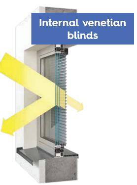
Due to the use of an internal blind only a small part of the solar energy is reflected from the glass, while the rest is absorbed into the room, emitting heat. This leads to the room overheating.
