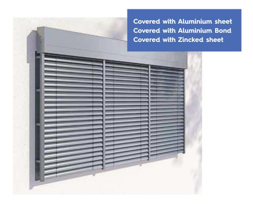
The self-supporting version of the venetian blind has been designed mainly for façade installation in buildings with large glazing. Due to the clever design the guide channels are the load-bearing element of the system. They transfer the entire weight to the façade columns. The product provides for the possibility of modular installation in one cassette up to 6000 mm. Max. dimensions are:  $4500 \times 4000$  mm (max. surface  $18 \text{ m}^2$ ).
