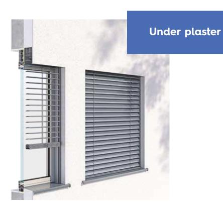
The venetian blind in the BX under plaster version was designed mainly for easy and quick installation in newly built buildings. The cover box is a ready-made element and is made of bent aluminium sheet. It can be fitted with a plaster foundation on both sides, allowing any plasterwork to be carried out. The system has dedicated guide channels to facilitate on plaster mounting in two sizes. Max. dimensions are  $4500 \times 4000$  mm (max. surface  $18 \text{ m}^2$ ).
