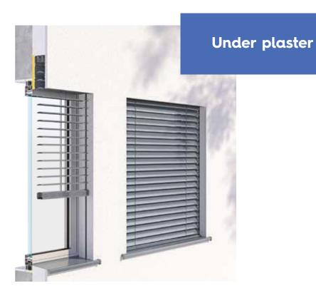
The under plaster version of the venetian blind is designed for installation in new buildings or exisiting ones if the necessary changes are introduced within the lintel. The protective cassette is made of extruded aluminium and has a special plaster support, allowing the plasterwork with any finishing material. Max. dimensions are:  $4500 \times 4000$  mm (max. surface  $18 \text{ m}^2$ ).
